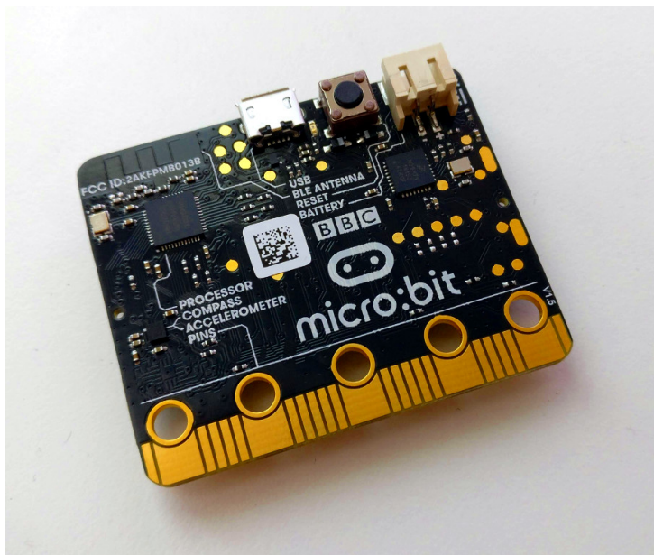
Kuva 2: Microbit from behind. On the top are usb-connector, reset button and the power connector.
